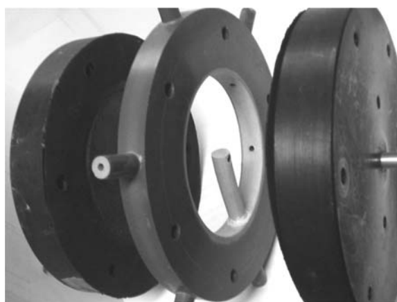
Fig. 2. View of the cell compartments, showing inlet and outlet connectors.
